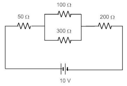
a. Calculate the equivalent resistance of the circuit.
