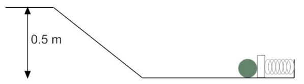
The spring, with a spring force constant of 100 N/m, is compressed 20 cm. The ball has a mass of 1 kg.
