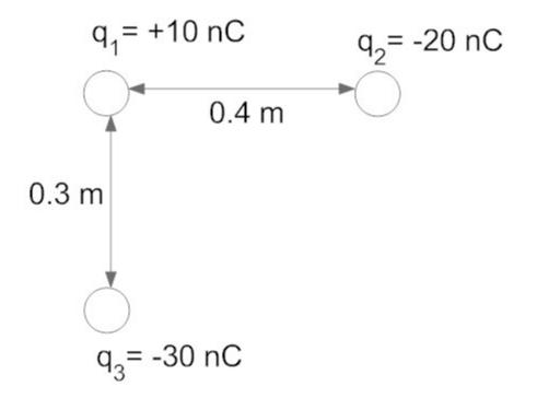
Calculate the net electrostatic force on  $q_3$ .
